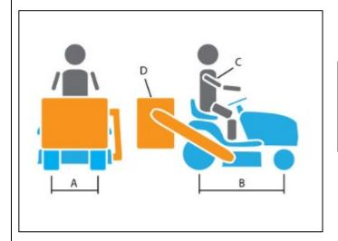
The **stability** of a ride on mower is affected by a) track width, b) wheelbase, c) position of operator and d) accessories fitted e.g. sun canopy.
