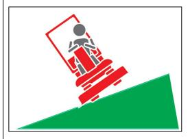
A **Front Mower** is at the highest risk of overturning on its side when operating across a steep slope.
