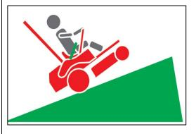
A **Zero Turn Mower** is at the highest risk of backflipping when operating up a steep slope; the two wheel configuration means is has less traction than a 4-wheel drive ride on mower.
