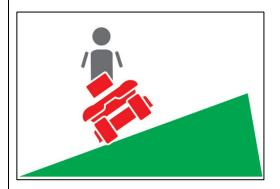
A **Traditional Ride on Mower** is at the highest risk of overturning on its side when operating across a steep slope; traditional ride on mowers are not fitted with a roll protective structure and should not be used on steep slopes.
